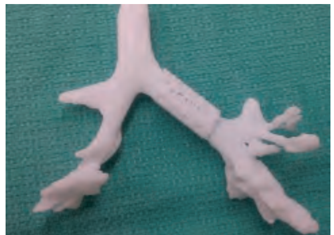
A 3D model of Kaiba’s windpipe with the “printed” splint in place.
